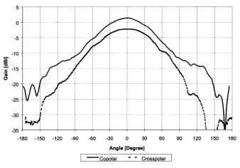
Fig. 4. Experimental E-plane gain.
