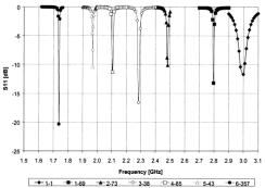
Fig. 1. Evolution of the patch input reflection coefficient.
