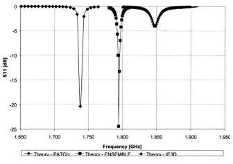
Fig. 3. Theoretical input reflection coefficient.
